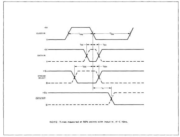
AC CHARACTERISTICS  $~V_{CC}$  = +5V  $^{\pm}$  5%;  $V_{GG}$  = -12V  $^{\pm}$  5%;  $T_{A}$  = 0° to +70°C
