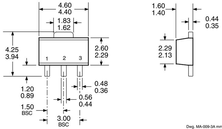
NOTES: 1. Tolerances on package height and width represent allowable mold offsets. Dimensions given are measured at the widest point (parting line).
