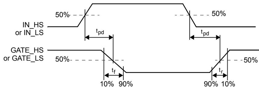
Figure 4. Timing Characteristics
