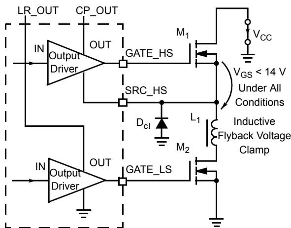
Figure 12. Gate Protection and Flyback Voltage Clamp
