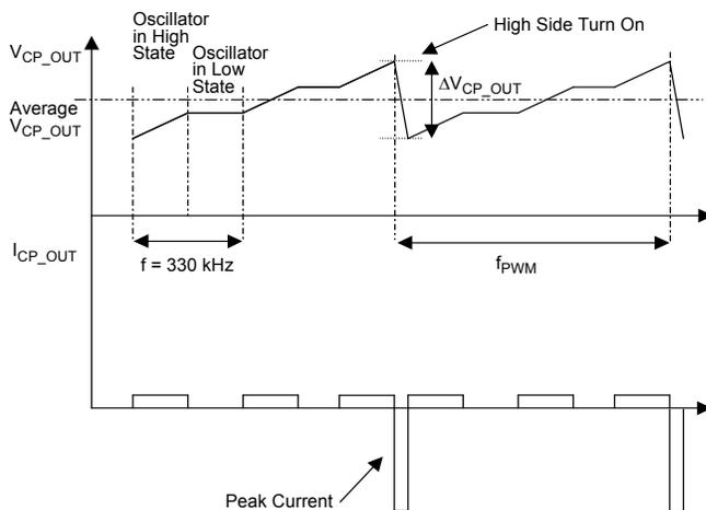
Figure 11. Simplified C<sub>CP\_OUT</sub> Current and Voltage Waveforms
