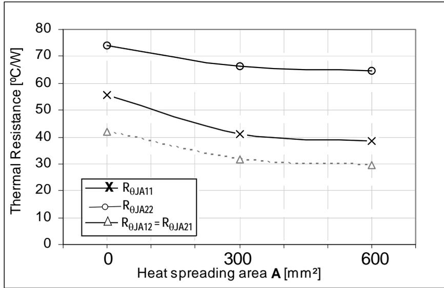
Figure 3. Device on Thermal Test Board R<sub>θJA</sub>
