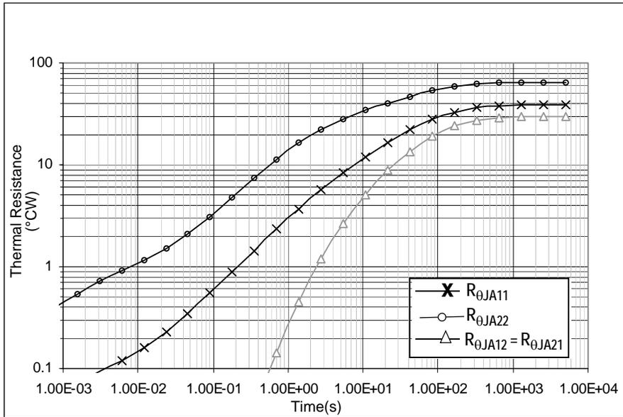
Figure 4. Transient Thermal Resistance R<sub>θJA</sub> (1.0 W Step Response)
