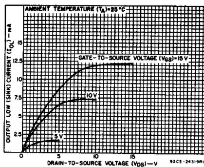
Fig. 7 - Minimum n-channel output low (sink) current characteristics.
