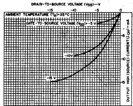
Fig. 9 — Minimum p-channel output high (source) current characteristics.
