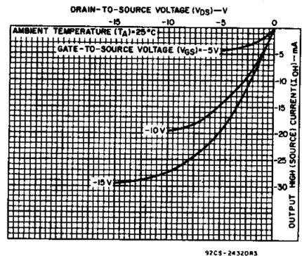
Fig. 8 - Typical p-channel output high (source) current characteristics.
