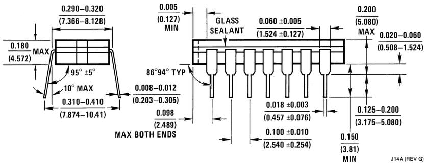
**14 Lead Ceramic Dual-In-Line Package (D)**
