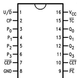
**Figure 2. Pin Assignment for DIP and Flatpak**
