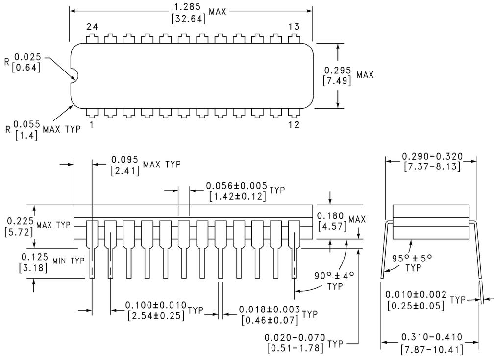
**24-Lead Ceramic Dual-In-Line Package (D)**
