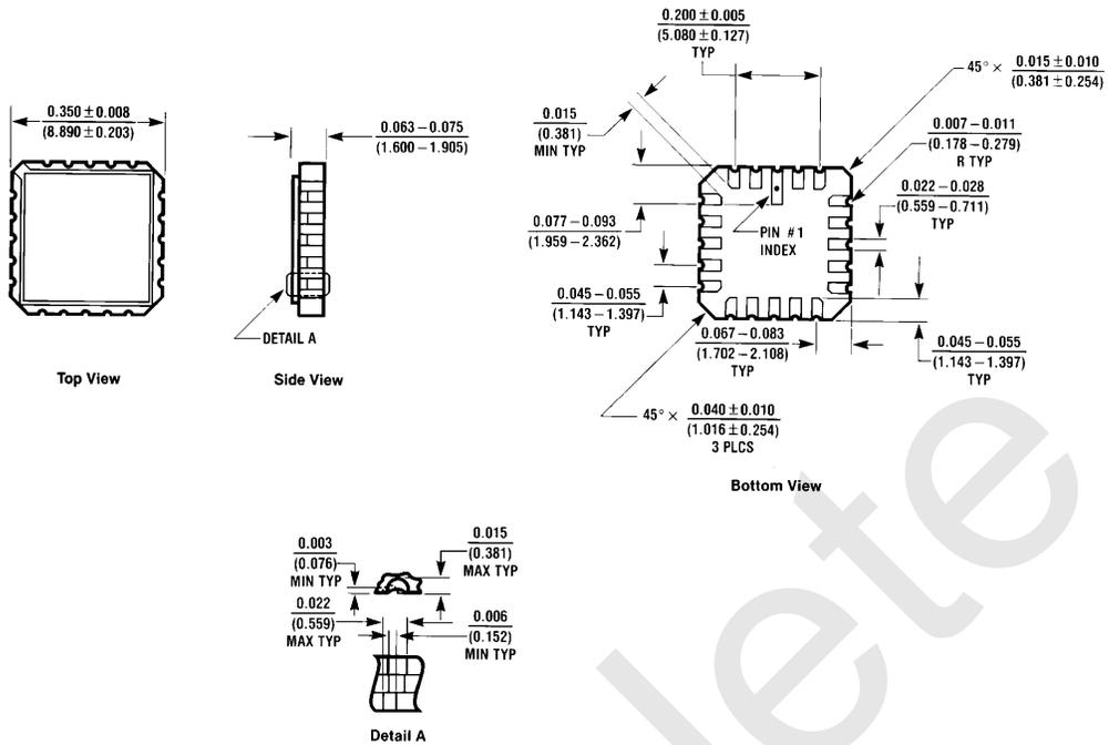
**20-Lead Ceramic Leadless Chip Carrier (L)
