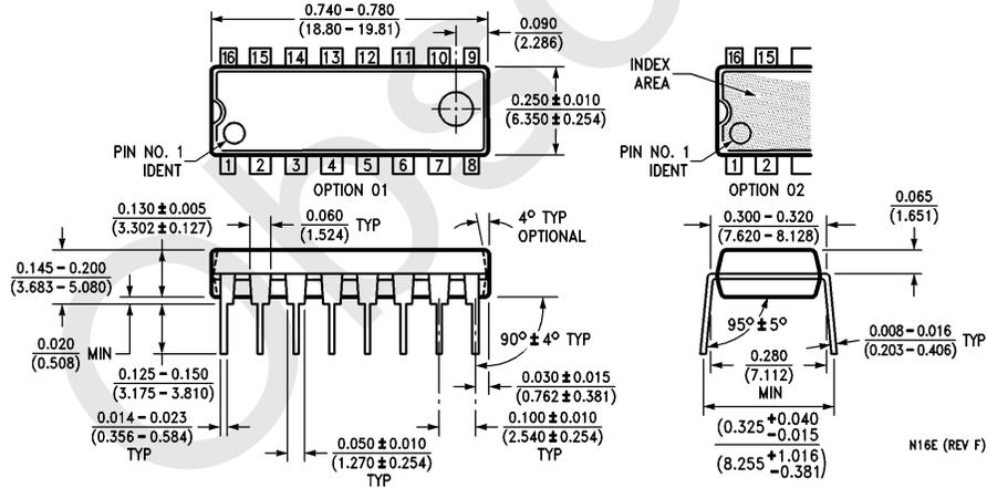
**16-Lead (0.300" Wide) Molded Dual-In-Line Package (P)
