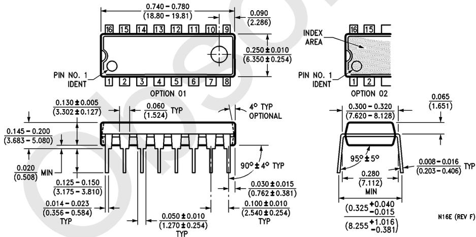
**16-Lead Molded Dual-In-Line Package (N)**
