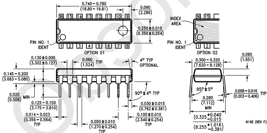
**16-Lead Molded Dual-In-Line Package (N)**
