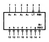
V<sub>CC</sub> = Pin 16 GND = Pin 8
