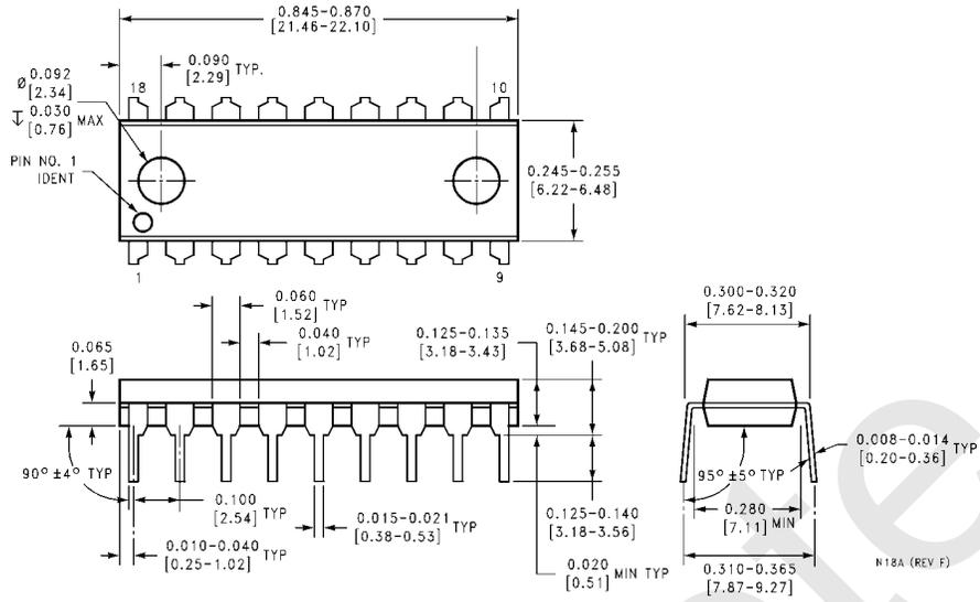
**18-Lead (0.300" Wide) Molded Dual-In-Line Package (P)**
