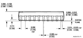
Figure 2. 20-Lead Small Outline Integrated Circuit (SOIC), JEDEC MS-013, 0.300" Wide Package Number M20B
