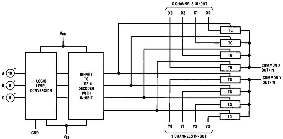
74VHC4051, 8-Channel Analog Multiplexer 74VHC4052, Dual 4-Channel Analog Multiplexer
