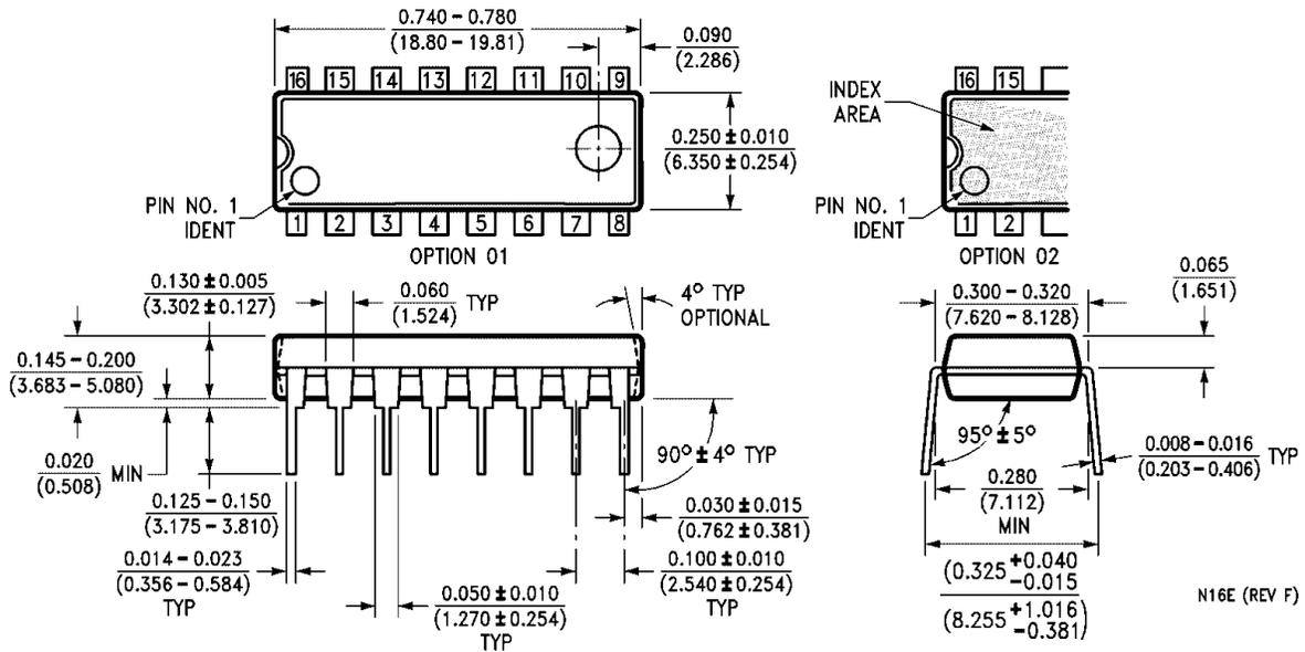
Figure 12. 16-Lead Plastic Dual-In-Line Package (PDIP), JEDEC MS-001, 0.300" Wide
