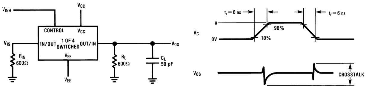
Figure 7. Crosstalk: Control Input to Signal Output
