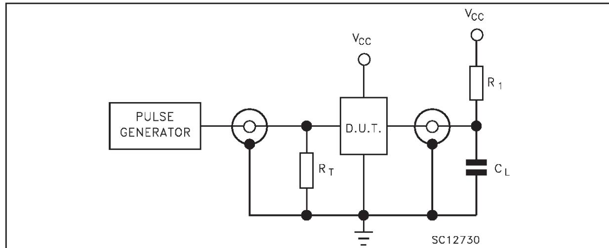
$C_L = 15/50\text{pF}$  or equivalent (includes jig and probe capacitance) $R_L = R_1 = 1\text{K}\Omega$  or equivalent $R_T = Z_{OUT}$  of pulse generator (typically  $50\Omega$ )
