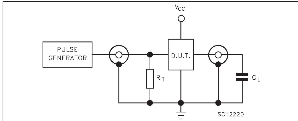
$C_L = 15/50 \text{ pF}$  or equivalent (includes jig and probe capacitance) $R_T = Z_{OUT}$  of pulse generator (typically  $50\Omega$ )
