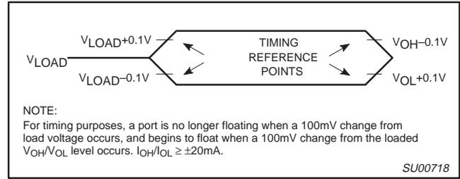
**Figure 20. Float Waveform**
