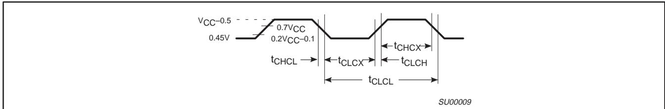
**Figure 24. Clock Signal Waveform for  $I_{CC}$  Tests in Active and Idle Modes**
