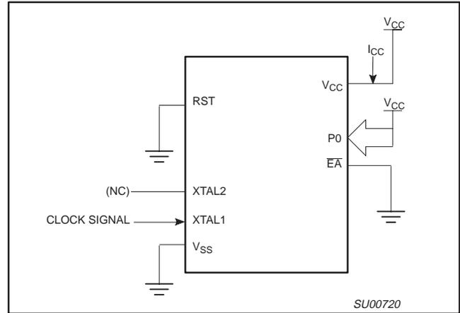
**Figure 23.  $I_{CC}$  Test Condition, Idle Mode**
