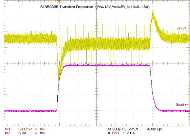
Figure 6. PWM Load Transient (0 to 15A)
