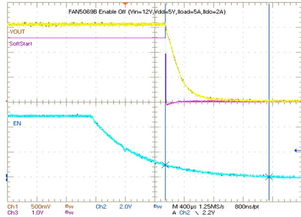
**Figure 13. Enable OFF ( $I_{PWM} = 5A$ )**
