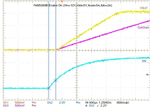
**Figure 12. Enable ON ( $I_{PWM} = 5A$ )**
