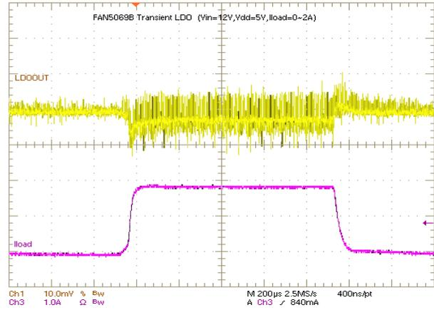
Figure 7. LDO Load Transient (0 to 2A)
