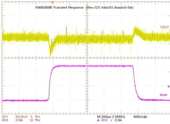
Figure 4. PWM Load Transient (0 to 5A)
