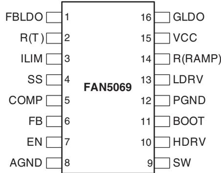
Figure 2. Pin Assignment
