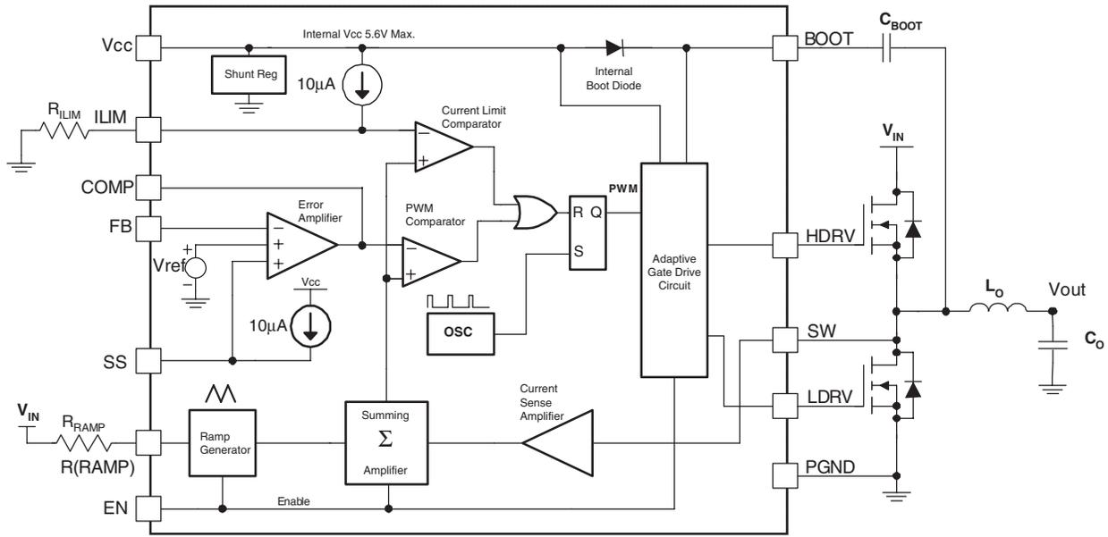
Figure 20. Block Diagram
