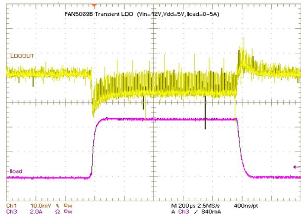
Figure 8. LDO Load Transient (0 to 5A)
