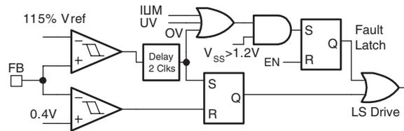
Figure 21. Over-Voltage Protection
