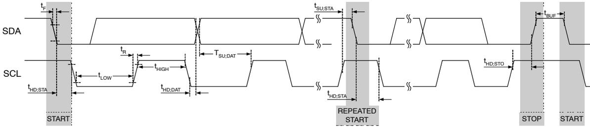
Figure 3. I<sup>2</sup>C Interface Timing for Fast Plus, Fast, and Slow Modes
