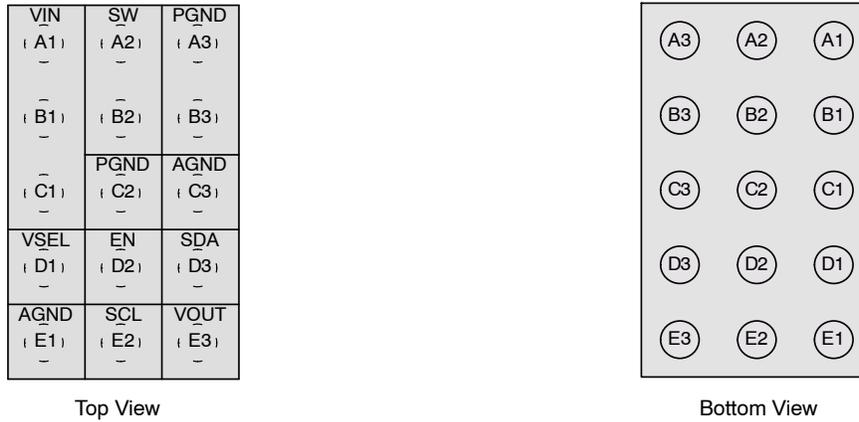
**Figure 2. Pin Configuration**
