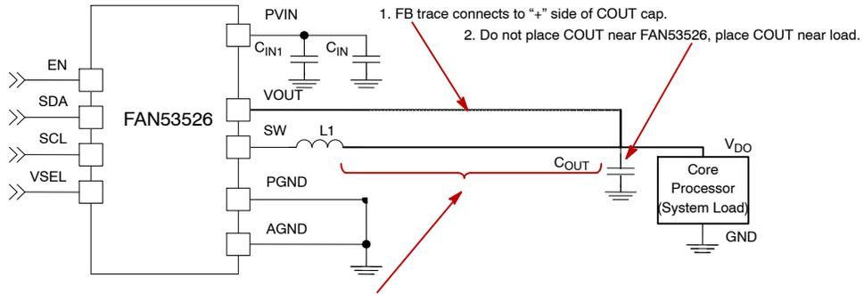
3. Maximum trace resistance between the inductor and the load should not exceed 30m $\Omega$ . For a 20 mils wide PCB trace with 0.5mils thickness using 2oz. Copper, a length of 0.5 inches gives a resistance of 24.3m $\Omega$ .
