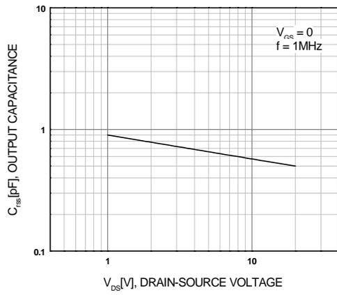
Figure 7.  $C_{RSS}$ - $V_{DS}$
