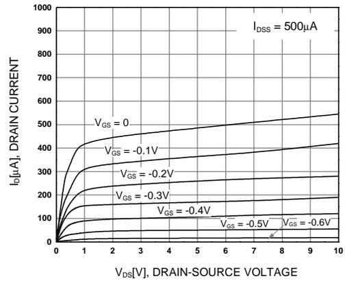
Figure 2.  $I_D$ - $V_{DS}$
