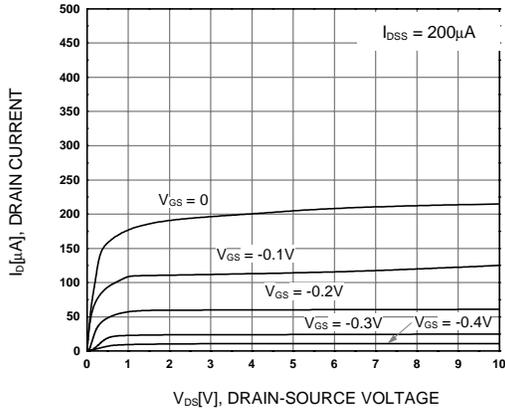
Figure 1.  $I_D$ - $V_{DS}$
