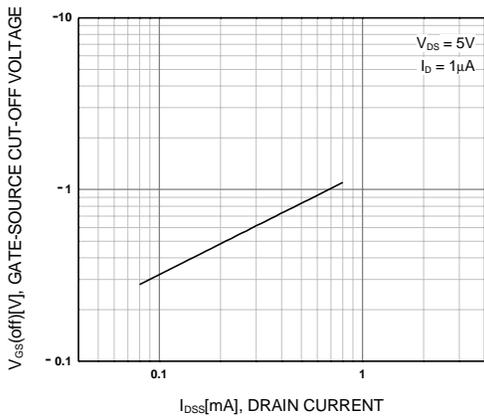
Figure 5.  $V_{GS(off)}$ - $I_{DSS}$
