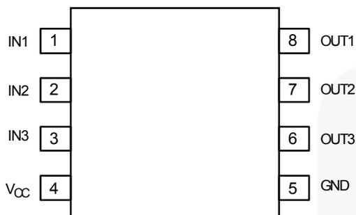
Figure 2. 8-Pin SOIC
