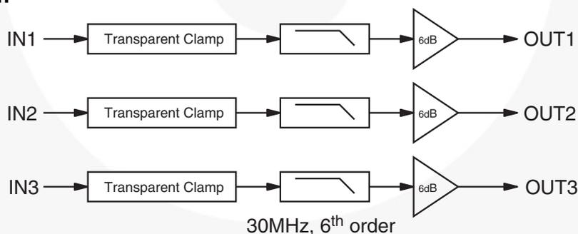
Figure 1. Block Diagram
