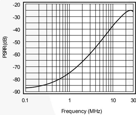
Figure 5. PSRR vs. Frequency; No Bypass Caps
