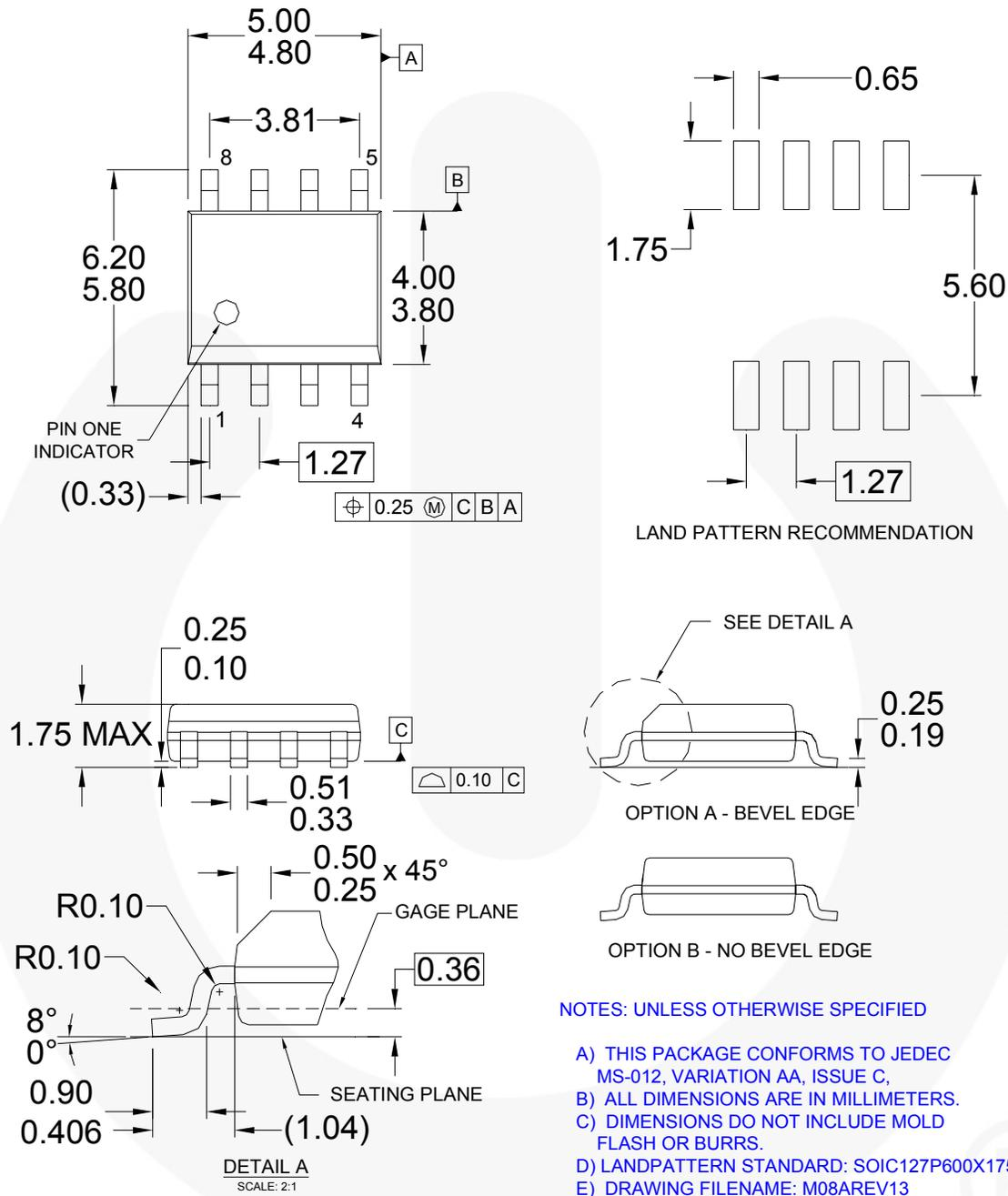
**Figure 18. 8-Lead, Small Outline Integrated Circuit (SOIC) Package**
