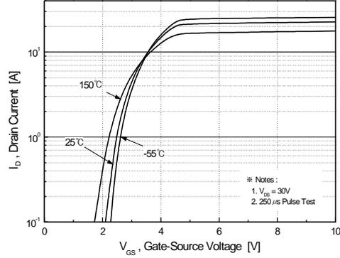
**Figure 2. Transfer Characteristics**
