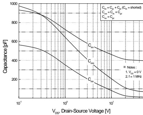
**Figure 5. Capacitance Characteristics**
