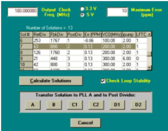
For a 100MHz output, the VCO should ideally operate at a higher frequency, and the Reference and Feedback Dividers should be as small as possible. In this example, highlight Solution #7. Notice the VCO operates at 200MHz with a Post Divider of 2 to obtain an optimal 50% duty cycle.
