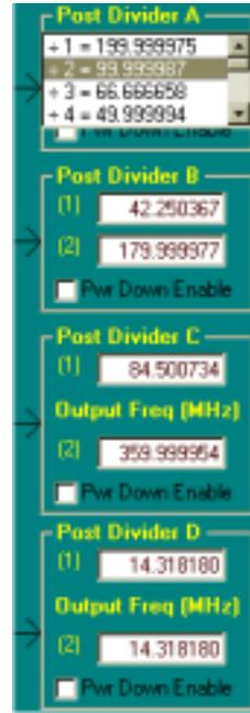
Click on PLL C1 to open the PLL screen. Set a desired frequency, however, now choose the Post Divider B as the output divider. Notice the Post Divider box has split in two (as shown in Figure 16). The Post Divider B box now shows that the divider is dependent on the setting of the SEL\_CD pin for as long as Mux B is the PLL C output.
