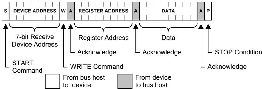
**Figure 6: Random Register Read Procedure**
