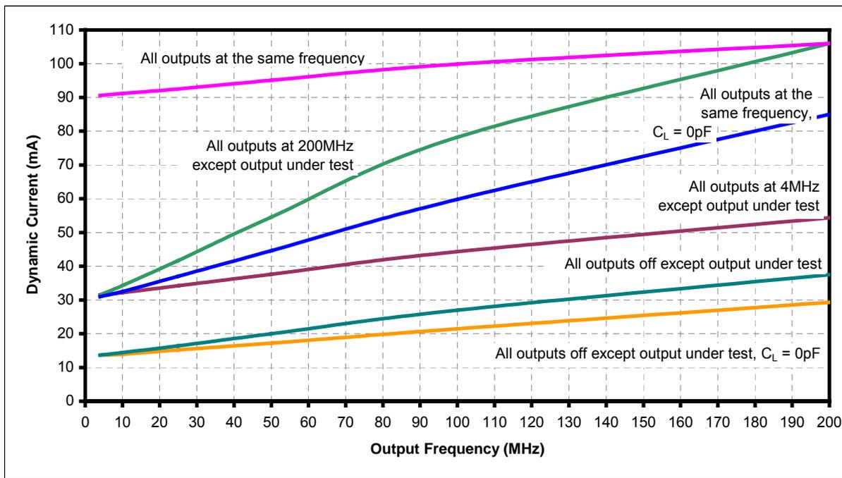
VDD = 3.3V; Reference Frequency = 27.00MHz; VCO Frequency = 100MHz, C<sub>L</sub> = 17pF except where noted
