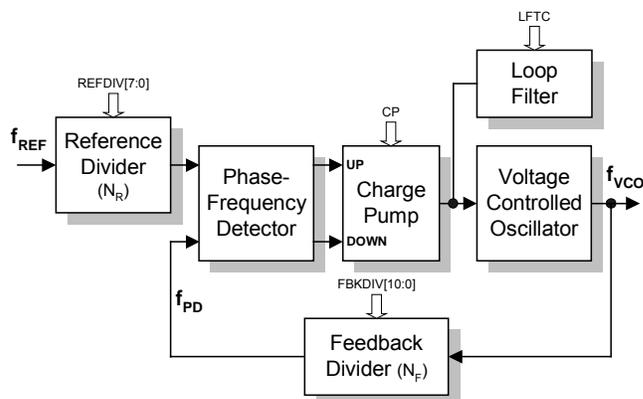
The PFD will drive the VCO up or down in frequency until the divided reference frequency and the divided VCO frequency appearing at the inputs of the PFD are equal. The input/output relationship between the reference frequency and the VCO frequency is
