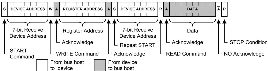
**Figure 7: Sequential Register Write Procedure**
