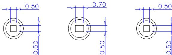
LEAD TYPE 1      LEAD TYPE 2      LEAD TYPE 3
