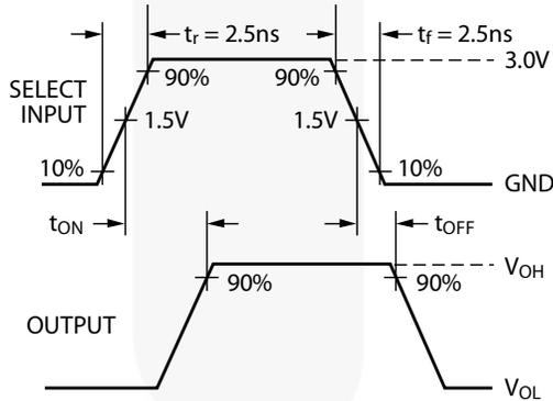
Figure 10. AC Waveforms
