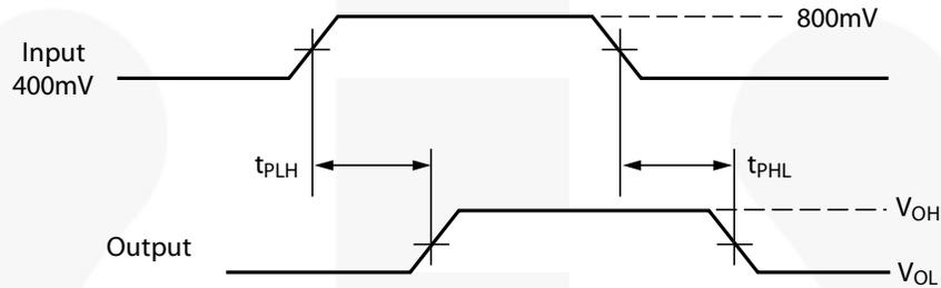
Figure 14. Propagation Delay
