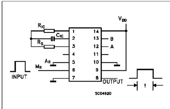
A positive MASTER RESET pulse clears the counters and latch. The output goes high and keeps up till the number of pulses, selected by A and B, are counted. This circuit is retriggerable and is as accurate as the input frequency. If a more accurate circuit is desired, an external clock can be used on pin 3. A set-up time equal to the width of the one shot output is required immediately following initial power up, during which time the output will be high.
