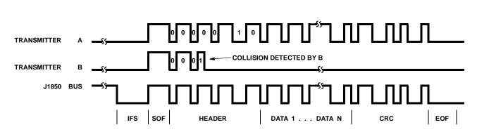
FIGURE 6. TWO NODES ARBITRATING FOR CONTROL OF J1850 BUS
