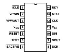
FIGURE 2. 14 PIN DIP AND SO TERMINAL ASSIGNMENTS
