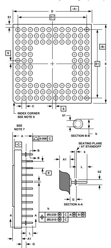
**G84.A** MIL-STD-1835 CMGA3-P84C (P-AC) 84 LEAD CERAMIC PIN GRID ARRAY PACKAGE
