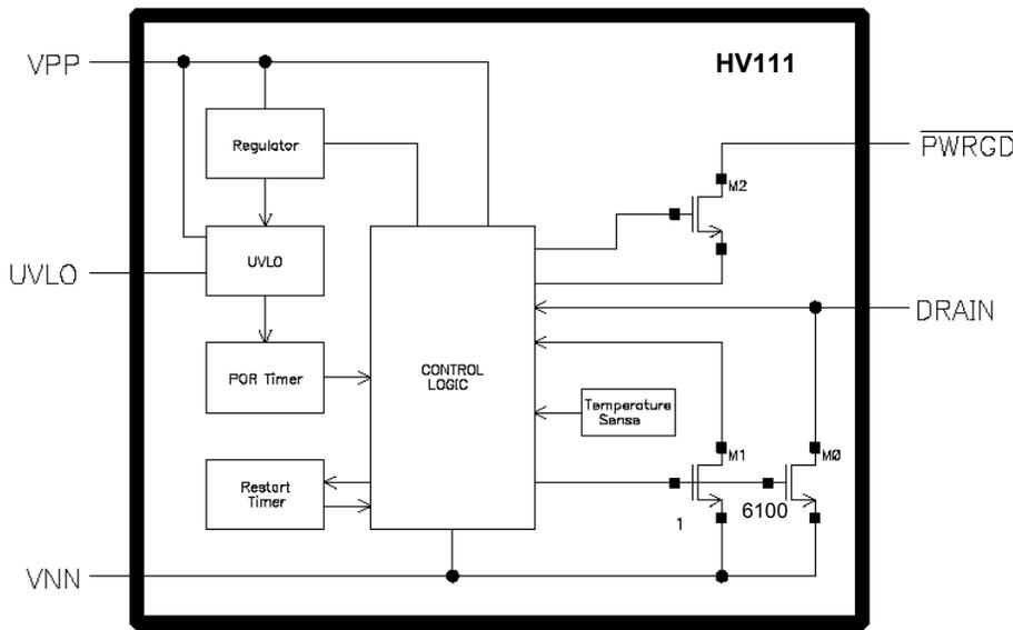
Figure 1 – Internal Blocks of HV111
