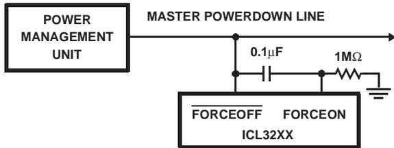
FIGURE 5. CIRCUIT TO ENSURE IMMEDIATE POWER UP WHEN EXITING FORCED POWERDOWN
