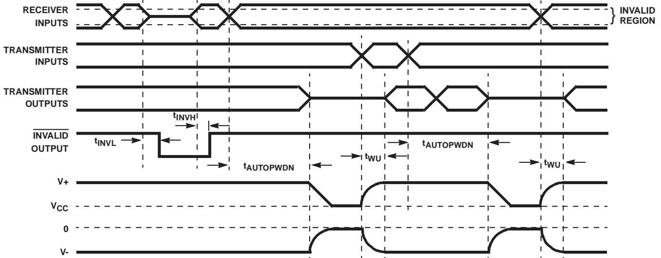
FIGURE 8. ENHANCED AUTOMATIC POWERDOWN, AND  $\overline{\text{INVALID}}$  TIMING DIAGRAMS
