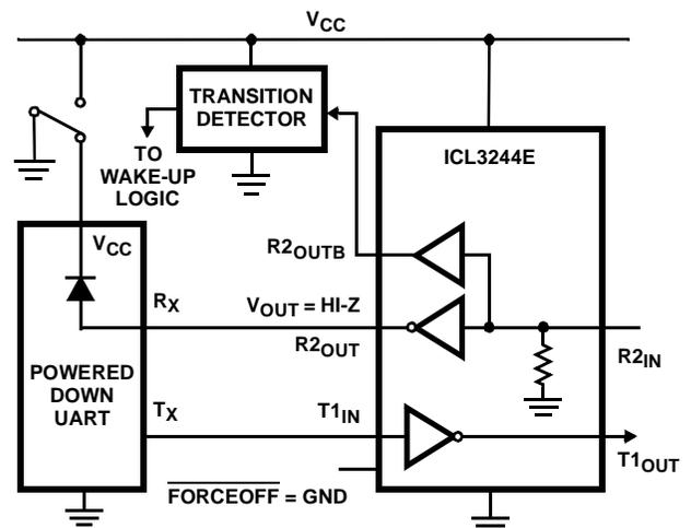
FIGURE 3. DISABLED RECEIVERS PREVENT POWER DRAIN
