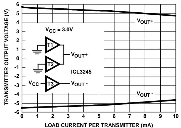
FIGURE 11. TRANSMITTER OUTPUT VOLTAGE vs LOAD CURRENT (PER TRANSMITTER, i.e., DOUBLE CURRENT AXIS FOR TOTAL V<sub>OUT+</sub> CURRENT)
