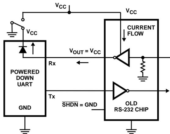
FIGURE 2. POWER DRAIN THROUGH POWERED DOWN PERIPHERAL
