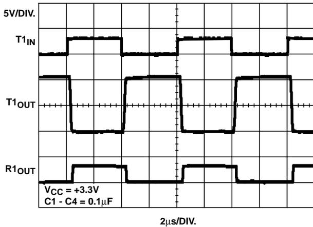
FIGURE 13. LOOPBACK TEST AT 250kbps ( $C_L = 1000\text{pF}$ )
