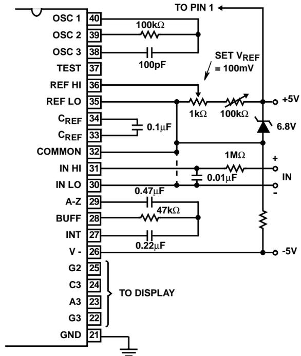
Since low TC zeners have breakdown voltages ~ 6.8V, diode must be placed across the total supply (10V). As in the case of Figure 14, IN LO may be tied to either COMMON or GND.
