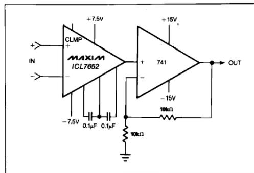
Figure 7. Using 741 to boost Output Drive Capability
