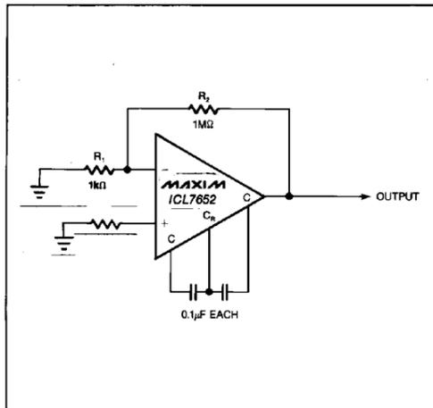
Figure 1. Maxim ICL7652 Test Circuit
