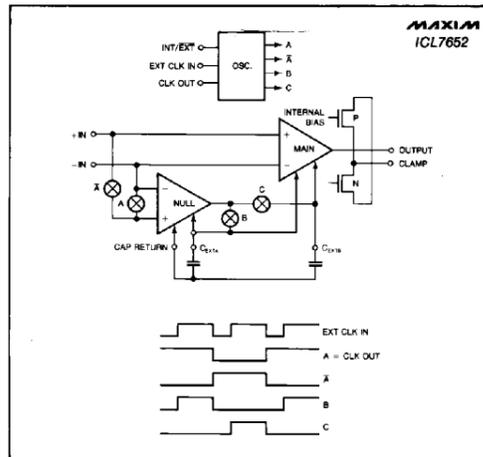
Figure 2. Maxim ICL7652 Block Diagram
