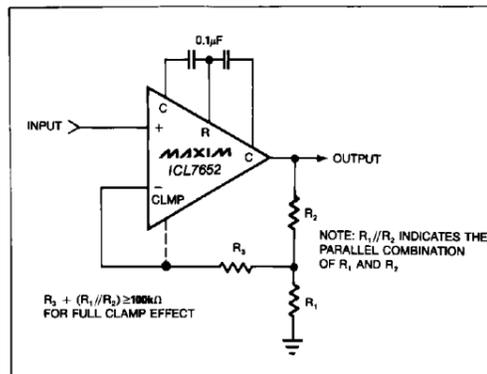
Figure 6. Non-Inverting Amplifier with Optional Clamp
