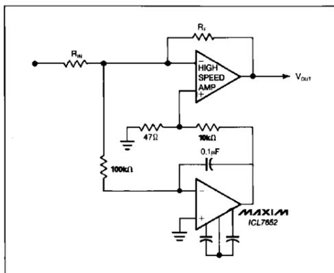
Figure 4. Nulling a High Speed Amplifier
