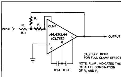
Figure 5. Inverting Amplifier with Optional Clamp
