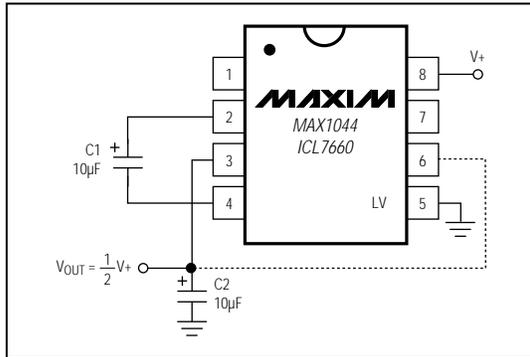
Figure 10. Voltage Divider
