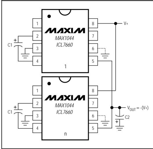
Figure 13. Paralleling MAX1044/ICL7660 to Reduce Output Resistance
