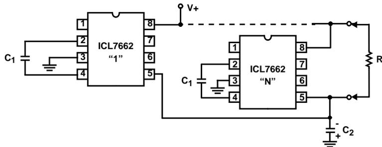
FIGURE 18. PARALLELING DEVICES
