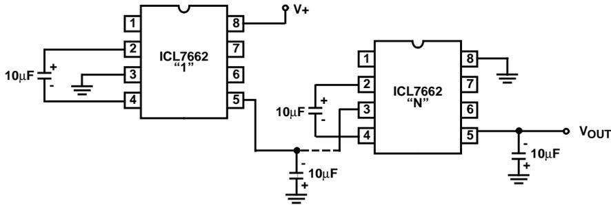
FIGURE 19. CASCADING DEVICES FOR INCREASED OUTPUT VOLTAGE
