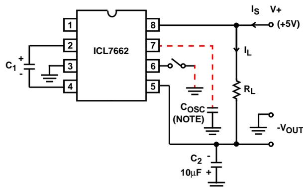
**NOTE:** For large value of  $C_{OSC}$  ( $> 1000pF$ ) the values of  $C_1$  and  $C_2$  should be increased to 100µF.
