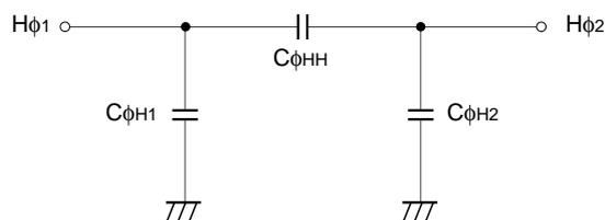
**Horizontal transfer clock equivalent circuit**
