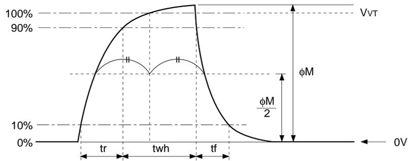
(2) Vertical transfer clock waveform
