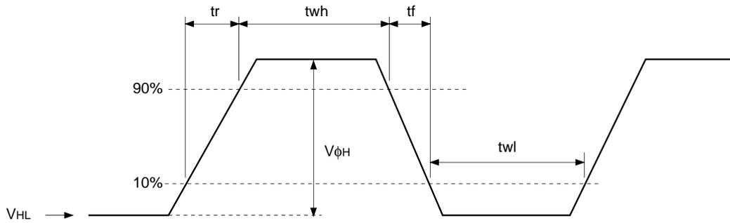
(4) Reset gate clock waveform
