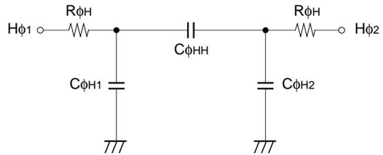
**Horizontal transfer clock equivalent circuit**
