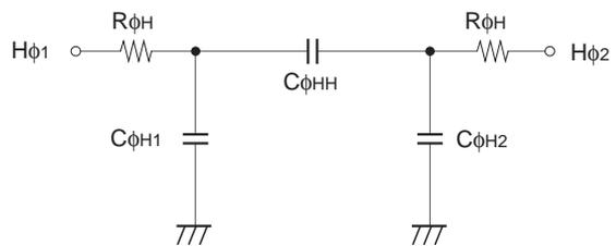
**Horizontal transfer clock equivalent circuit**
