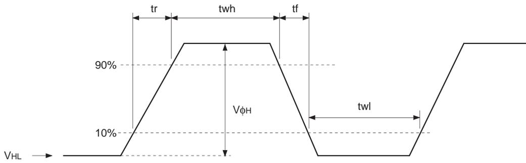
**(4) Reset gate clock waveform**
