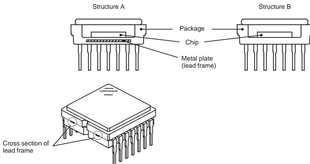
The cross section of lead frame can be seen on the side of the package for structure A.
