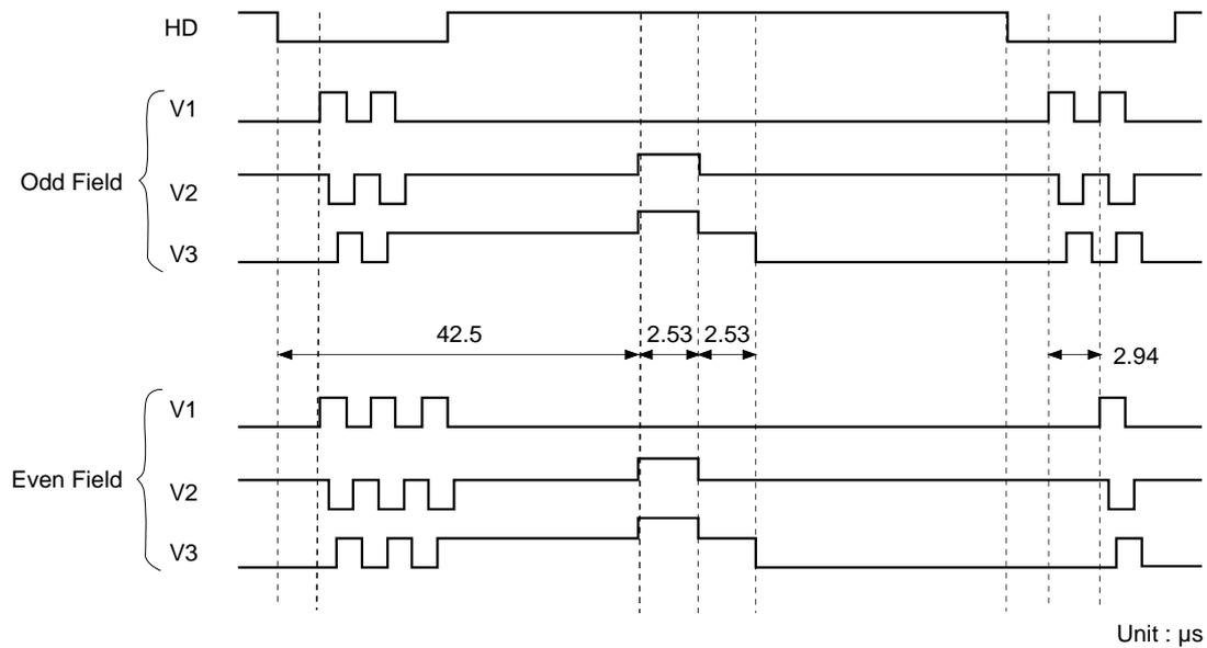
Drive Timing Chart (Vertical Sync) 1/60s interlaced mode
