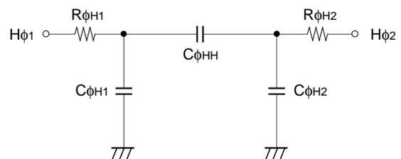
**Horizontal transfer clock equivalent circuit**
