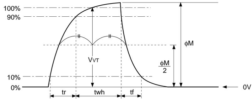
(2) Vertical transfer clock waveform
