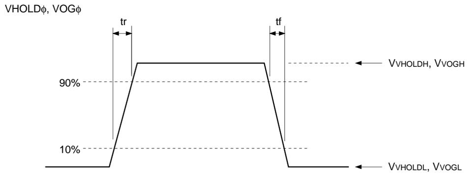
**(7) Inter-horizontal register transfer clock waveform**
