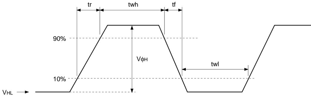
**(4) Reset gate clock waveform**
