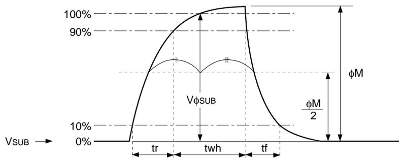
**(6) Vertical final stage accumulation clock waveform - Vertical final stage transfer clock waveform**
