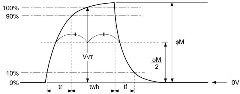
(2) Vertical transfer clock waveform
