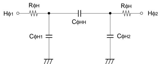
**Horizontal transfer clock equivalent circuit**
