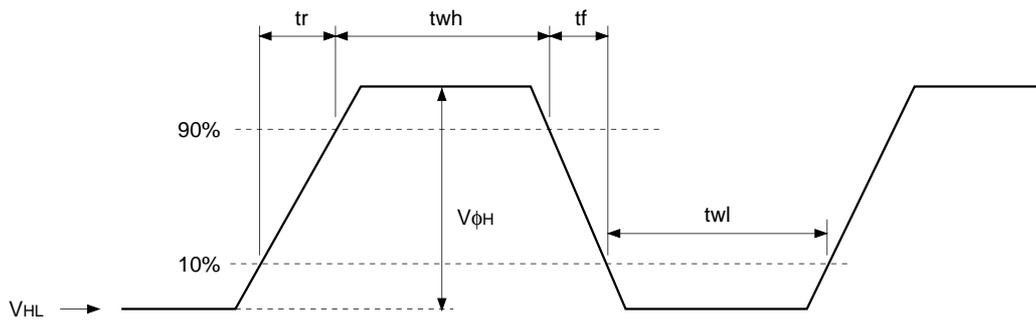
**(4) Reset gate clock waveform**
