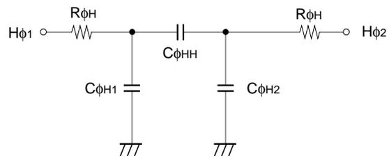
**Horizontal transfer clock equivalent circuit**
