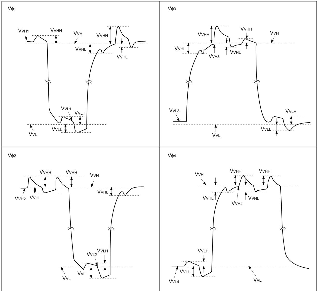
$$V_{VH} = (V_{VH1} + V_{VH2})/2$$
