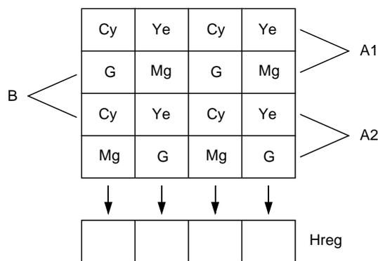
As shown in the left figure, fields are read out. The charge is mixed by pairs such as A1 and A2 in the A field. (pairs such as B in the B field)
