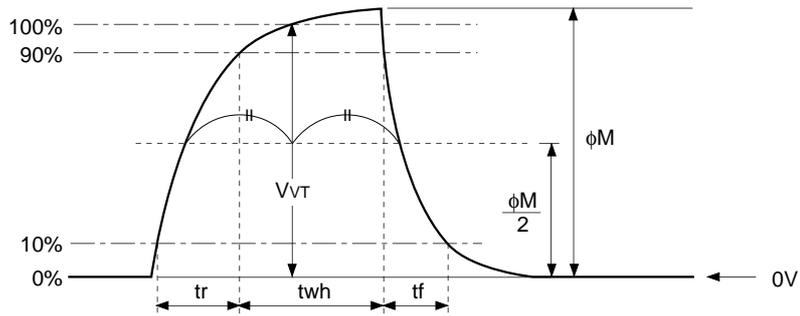
(2) Vertical transfer clock waveform
