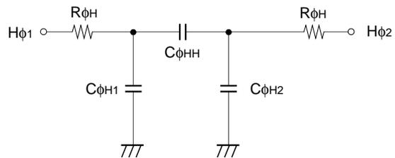
**Horizontal transfer clock equivalent circuit**
