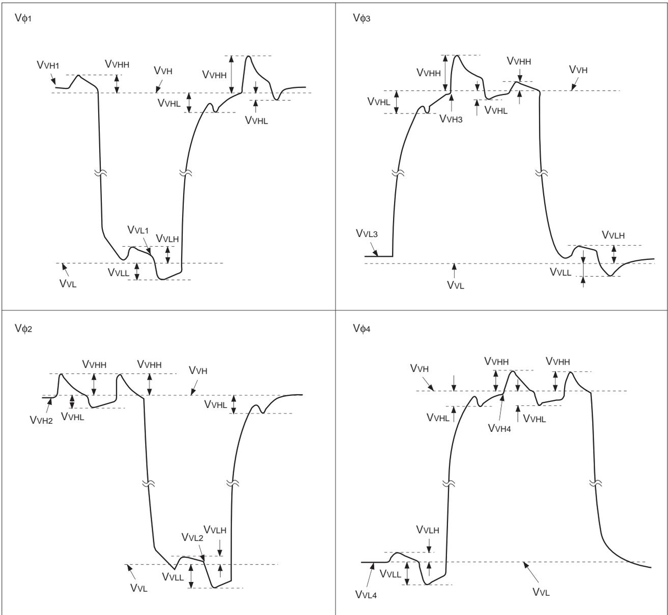
$$V_{VH} = (V_{VH1} + V_{VH2})/2$$
