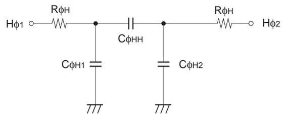
**Horizontal transfer clock equivalent circuit**
