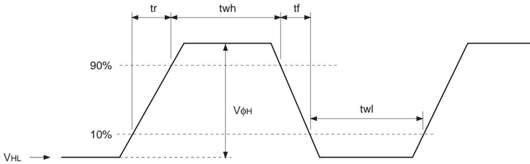
**(4) Reset gate clock waveform**
