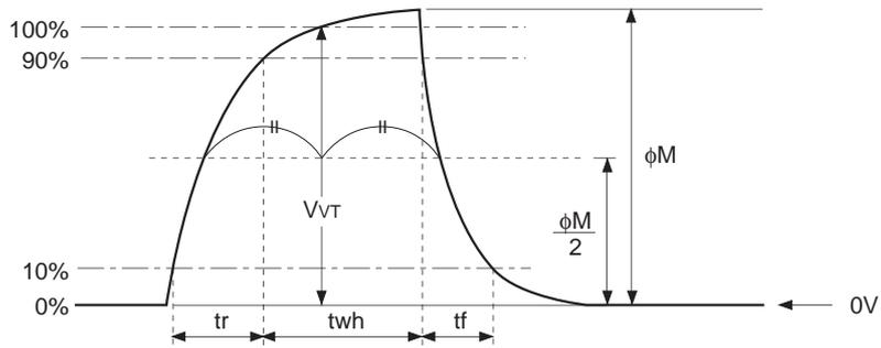
(2) Vertical transfer clock waveform
