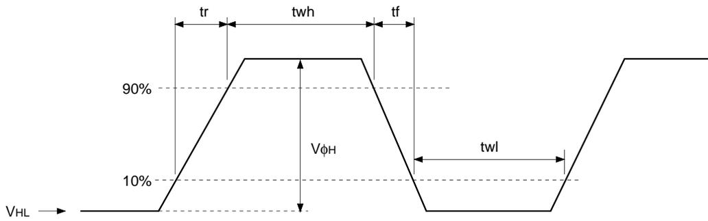
**(4) Reset gate clock waveform**
