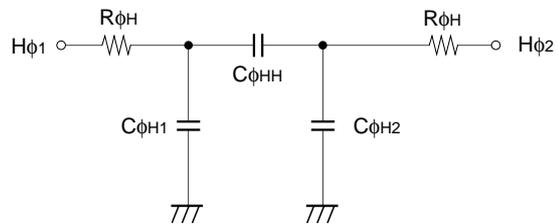
**Horizontal transfer clock equivalent circuit**
