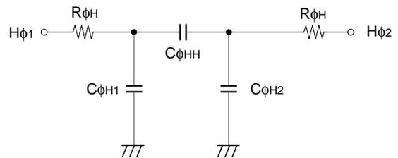
**Horizontal transfer clock equivalent circuit**
