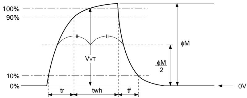
(2) Vertical transfer clock waveform
