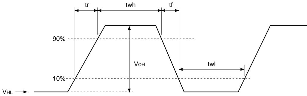
**(4) Reset gate clock waveform**
