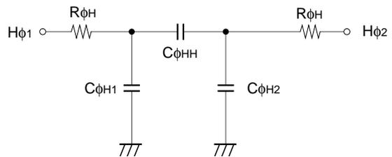
**Horizontal transfer clock equivalent circuit**
