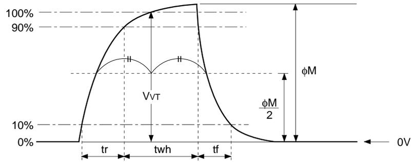
(2) Vertical transfer clock waveform
